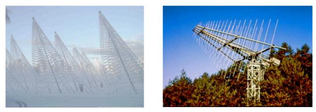
Figure 1. (Left) The Nançay Decameter Array consists in 144 helicoidal antennae divided in two left-handed and right-handed polarized subsets [1]. (Right) Historic log-periodic Yagi antenna in Nançay [2].
